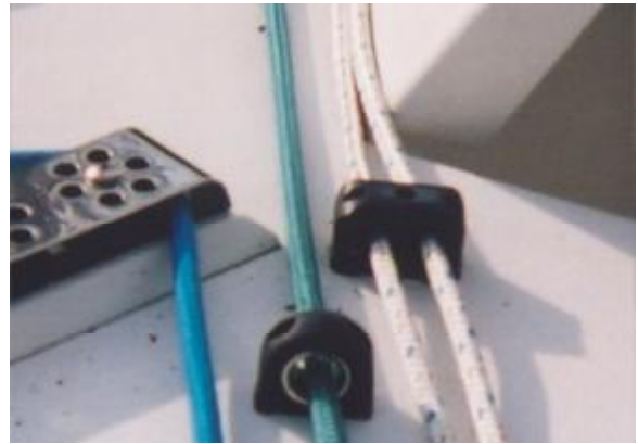
Three photos showing the furling line fairleads
