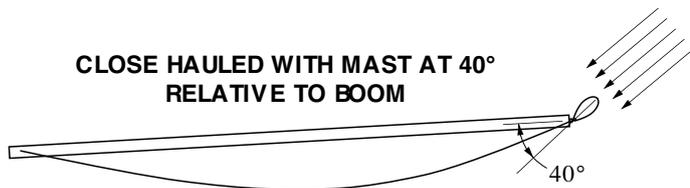
Avoid allowing the mast to rotate or swing back and forth, which can happen in light winds combined with waves, or when sailing off the wind with less sail pressure. This is usually prevented by having the mainsheet angled forward from the boom, which forces the boom forward to keep the mast rotated when pulled tight.
