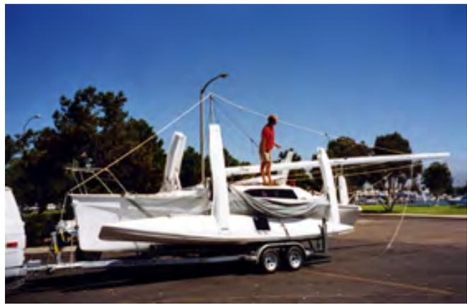
*Mast raising pole in position on an F-28 with winch line connected to jib halyard, ready to raise mast. Depending on design, take care that rotating mast is restrained once up so that it cannot topple forwards. This can be done by using the Corsair type Highfield Lever to connect shrouds to float chainplates, on older designs like F-28 and F-31. Modern designs like the F-22 or F-32 do not require these.*
