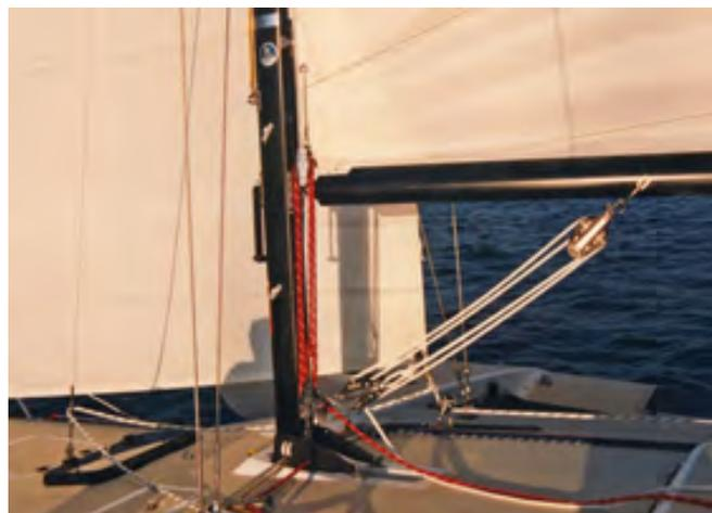
*Boom vang and Cunningham eye controls on an F-27 - Boom vangs are not used with rotating masts as they will restrict rotation*
