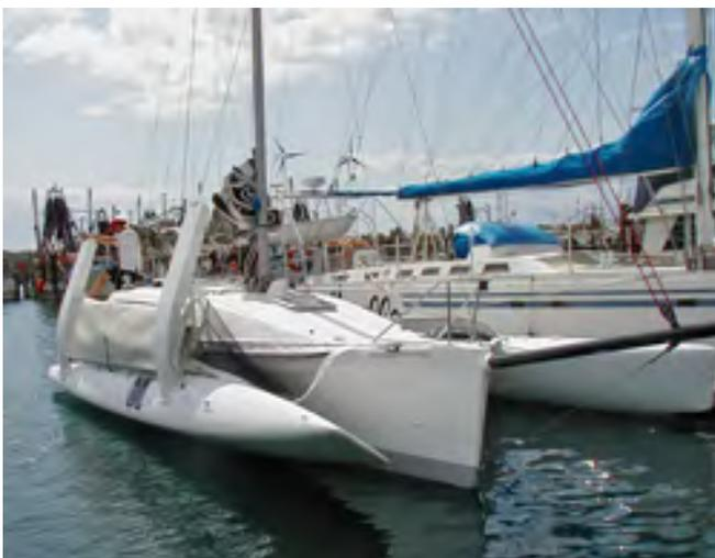
*F-33 being unfolded at dock. Folding is harder on larger designs with low profile beams and foot should be placed on Upper Folding Strut for leverage. May take two, or block and tackle assistance can be used if necessary - see later.*
