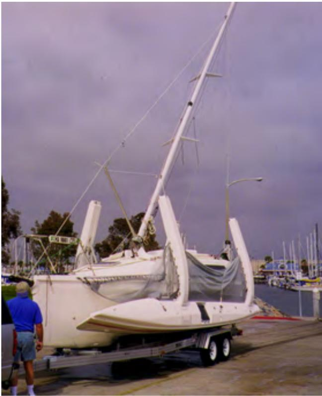
*F-31R/F-9R mast half way up, winch line just about to leave 'cradle' on raising pole. Watch float shroud turnbuckles if fitted, as they are easily snagged and bent. If one has to park on a side slope or be in a cross wind, then it is also a good idea to have someone on deck to stabilize mast or raising pole, or use extra side lines to stabilize pole, particularly on larger models.*
