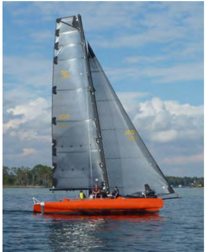
*Screacher being used to windward on F-32SR, while doing 16 knots in 8 knots of wind. Luff could be a little tighter, but very hard to do with that level of performance. A screacher is also be a great allround easy to use sail for cruisers.*
