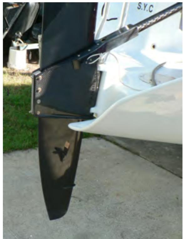
*A small fence fitted to an F-22R rudder blade*
