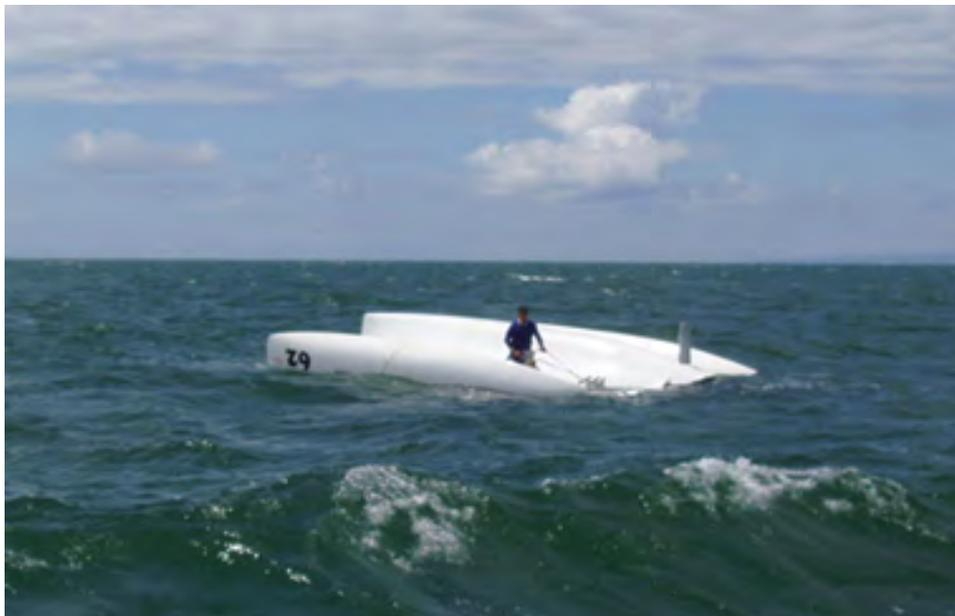
*Push it too far and this is what may happen - a capsized F-82 - note how high it is floating, the water level being around the bottom of the beams. Even in this position it remains a relatively easy and safe boat to be on. This is about as bad as it can get on an unsinkable multihull. The other option is this:*
