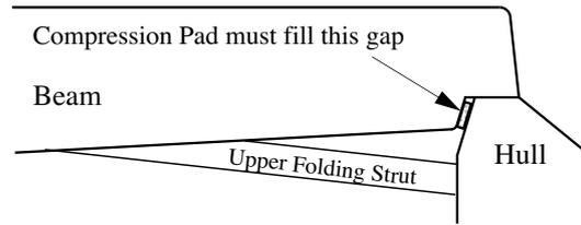
This would not cause a serious beam problem as the beams then simply move inboard to bear against the hull again. The boat is not threatened structurally. However, repairing an U.F.S. mounting point is difficult and expensive.
