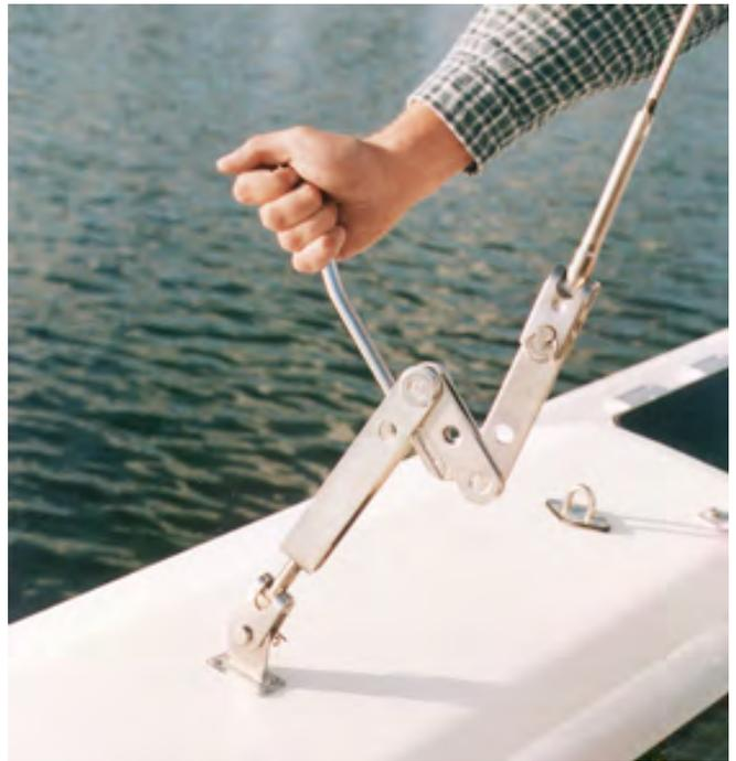
*Highfield lever being released on an older design to give enough slack in the float shroud for folding. Mast raising wires **must always be fitted prior to releasing shrouds**.*
