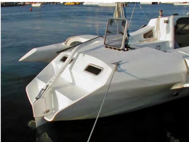
*F-33 daggerboard rudder, with blade fully down*
