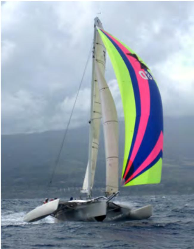
*Asymmetric spinnaker on an F-33R. Jib can also be flown inside by racers as shown for better performance*
