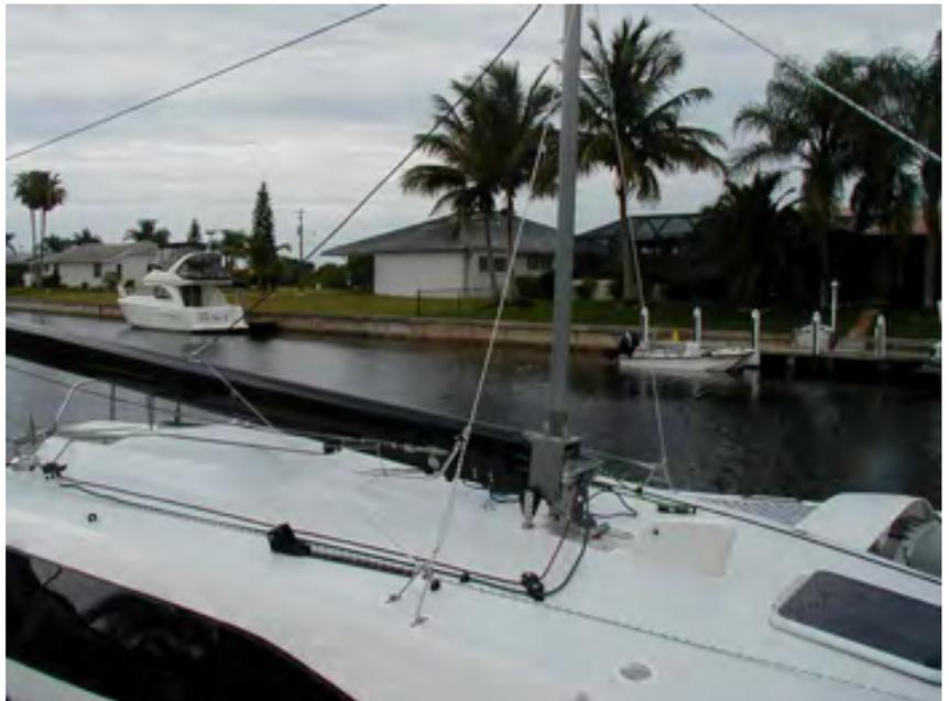
*Raising wire Deck Loops - these work well to anchor raising wires as they can fold down to be flush on deck when not in use. F-33 mast step with raising pole yoke shown above and below left. The same basic mast raising setup applies for both on trailer or on water mast raising.*
