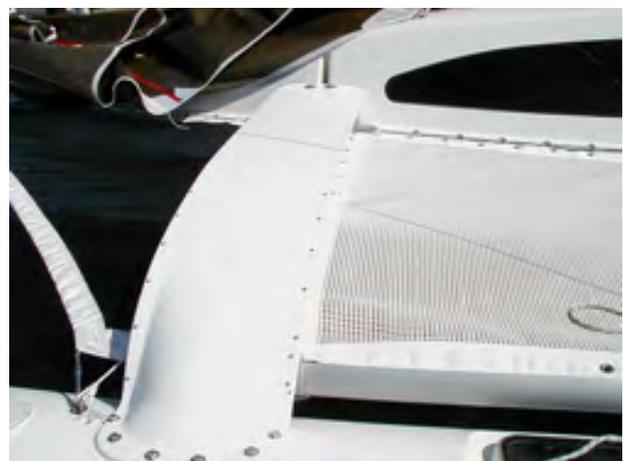
Wingnet gap and lashing to beam is completely covered on this F-33, making the nets safer. But still take care.
