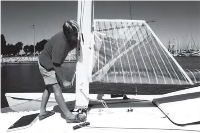
*F-28 Mainsail being roller furling. Note foot being used to control halyard.*
