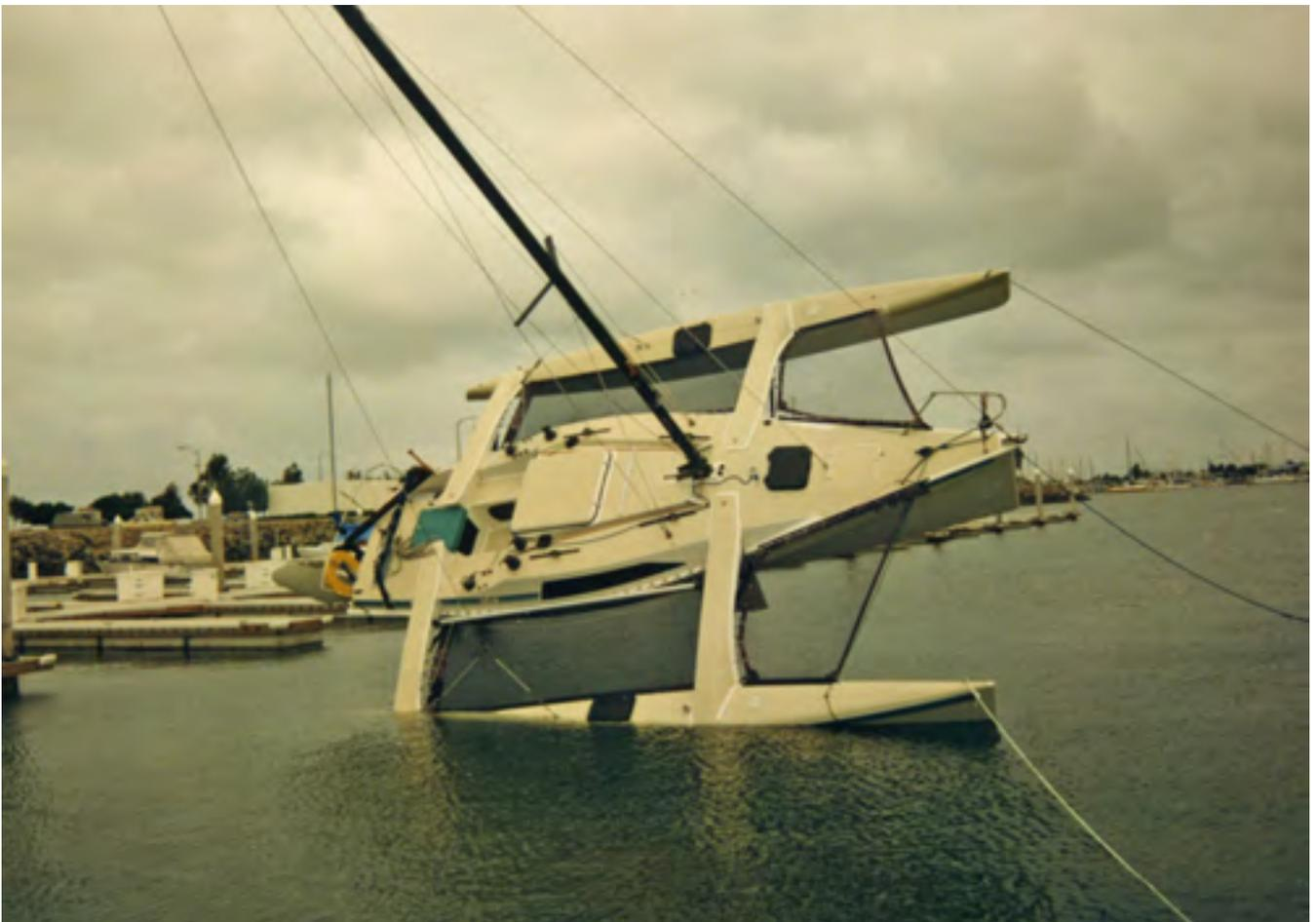
*This is **not** a safe angle of heel - go this far and you are probably gone! This F-27 is being pulled over to test stability.*
