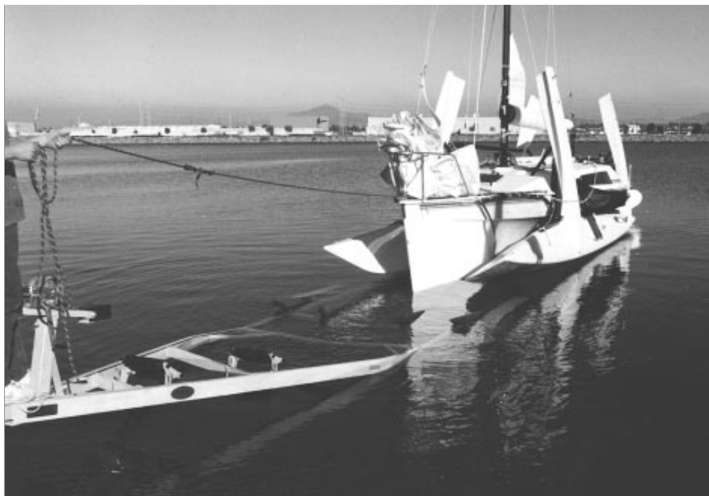
This is about the right position for the trailer when retrieving
